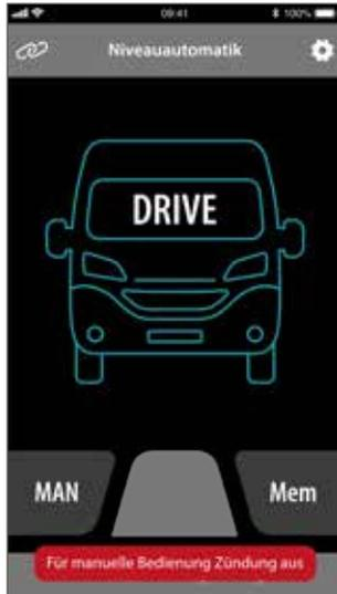
1. After the ignition is switched off, the system switches to after-run time manual mode.
