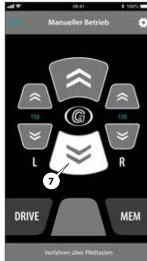
2. Press and hold the button (7). The air spring is lowered until the button is released.
