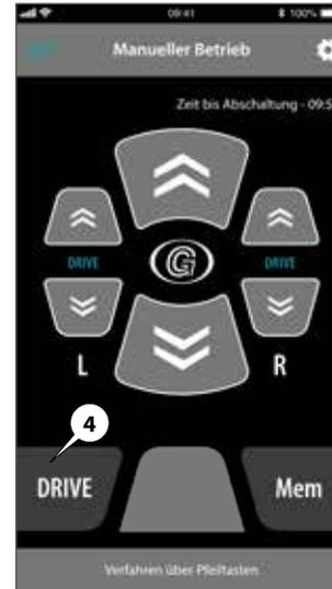
1. Press the Drive button (4) to establish the drive height
