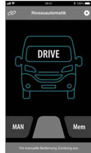
1. When the ignition is switched on, the screen switches to the **Automatic height control system** screen.
