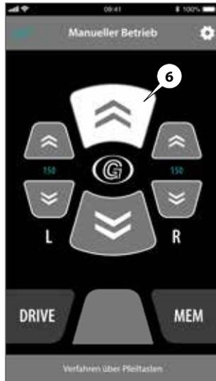
1. Press and hold the button (6). The air spring is lifted until the button is released.
